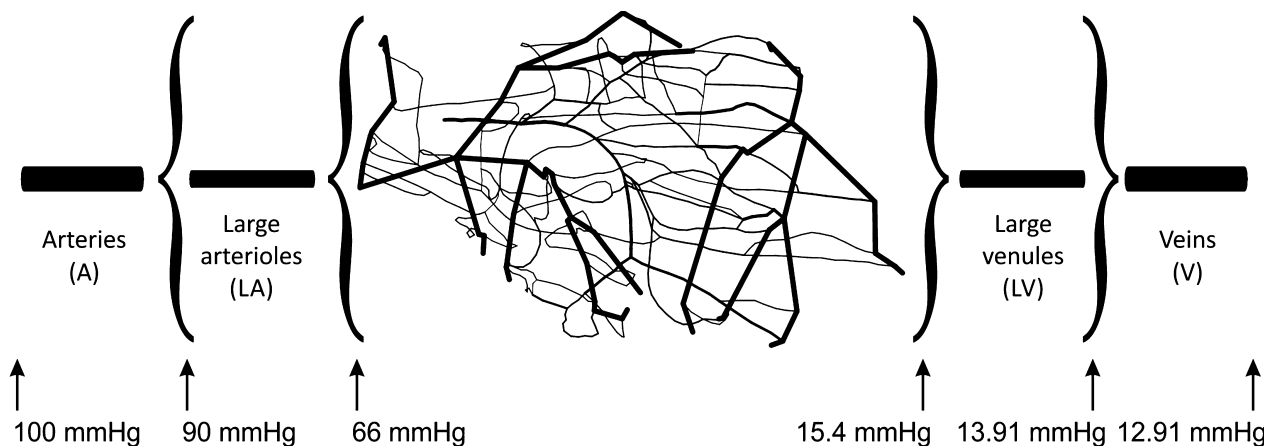
Figure 1. Schematic of the network model. A complete flow pathway through the circulation is formed by an experimentally observed microvascular network, with the addition of upstream and downstream segments representing arteries, large arterioles, large venules, and veins. The distribution of intravascular pressures is shown for the reference state of the network model.
