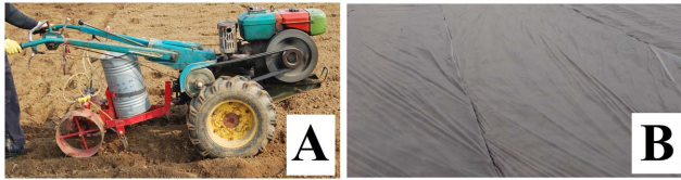
Figure 1. Application of Pic in field trials: (A) a manual injection machine was used to apply Pic in the soil; (B) the treatments were covered with PE or TIF film.
