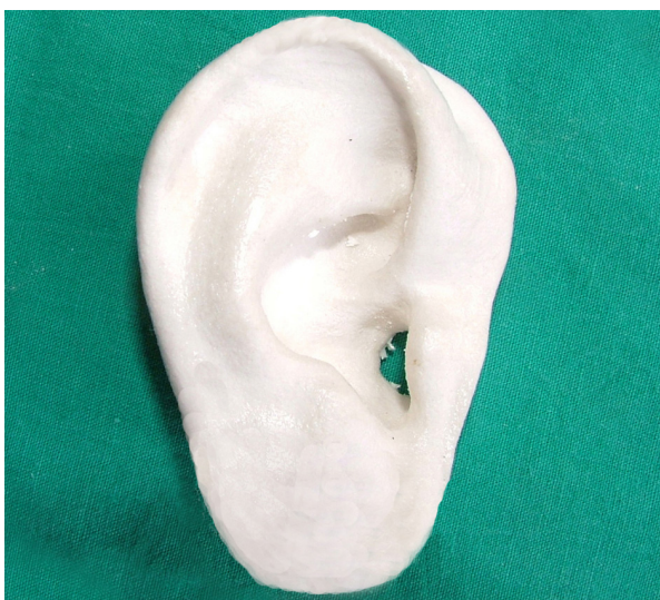
Figure 3. 3-D model obtained by 3-D ink-jet printing.
