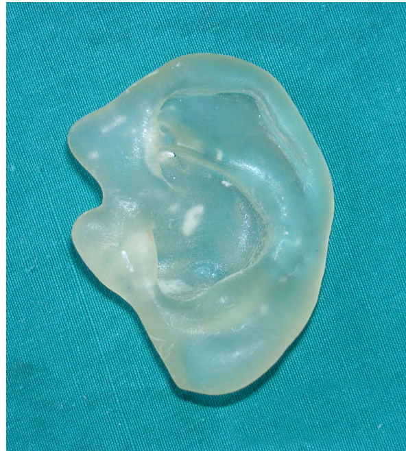
Figure 8. 3-D model obtained by stereolithography.
