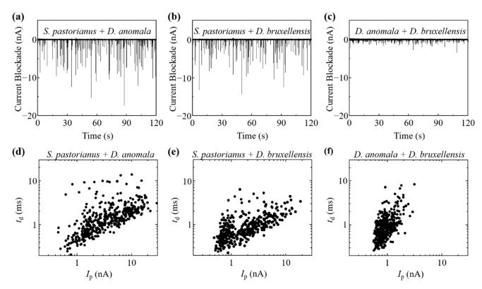
**Figure 3.** Electrical current record by RPM of each mixture of (a) *S. pastorianus* and *D. anomala*, (b) *S. pastorianus* and *D. bruxellensis*, and (c) *D. anomala* and *D. bruxellensis*.  $I_p$ - $t_d$  scatter plot on log-log graph by RPM of each mixture of (d) *S. pastorianus* and *D. anomala*, (e) *S. pastorianus* and *D. bruxellensis*, and (f) *D. anomala* and *D. bruxellensis*.
