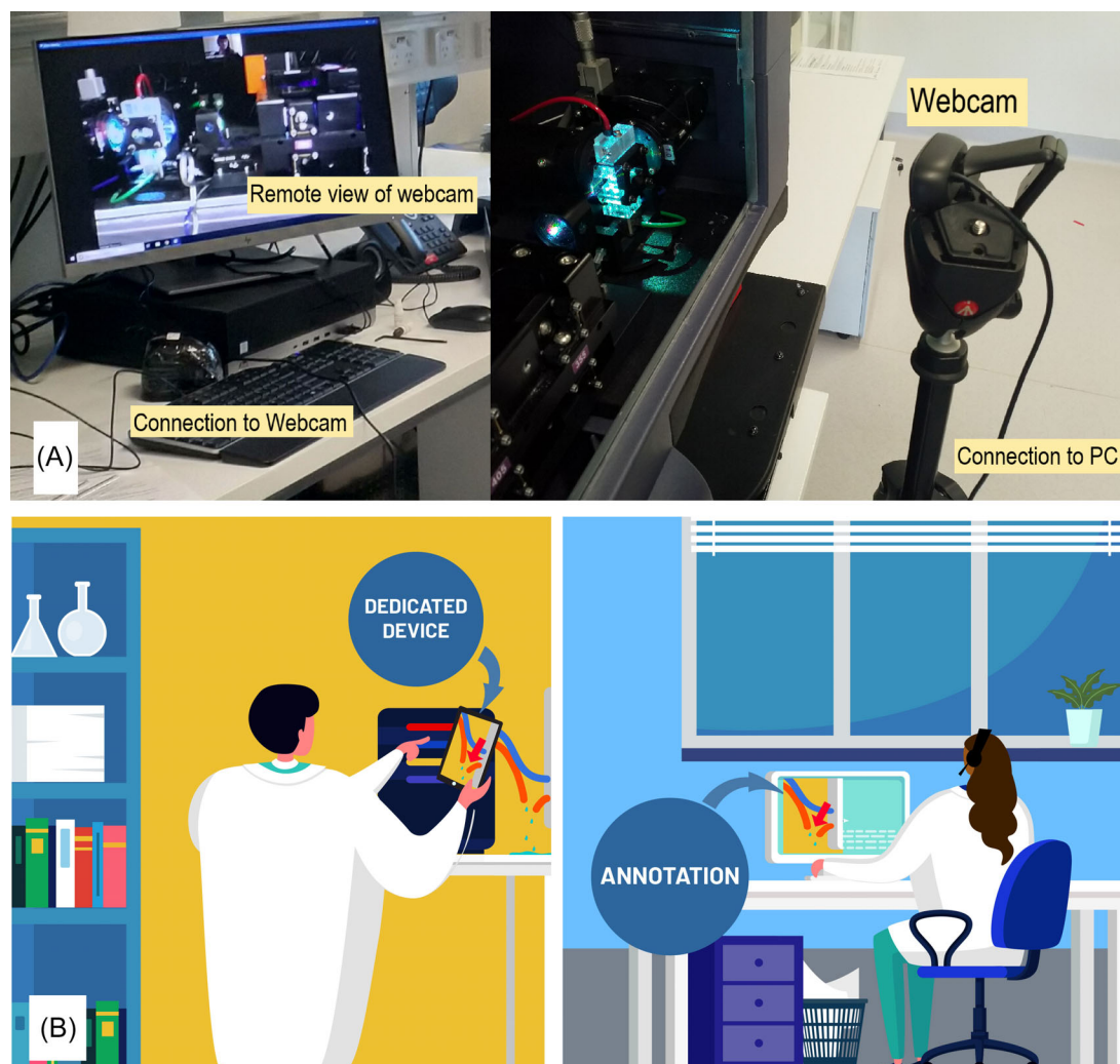
Fig 2. Remote support tools for instrument troubleshooting. (A) A webcam connected to the instrument workstation allows users and SRL staff to troubleshoot instrument hardware issues without the need for additional mobile devices. (B) Applications, such as TeamViewer Pilot, on a dedicated troubleshooting device enable SRL staff to remotely diagnose and troubleshoot issues using tools such as augmented reality. This is especially relevant when instrument workstations operate on outdated operating systems or are not networked. [Color figure can be viewed at wileyonlinelibrary.com ]
