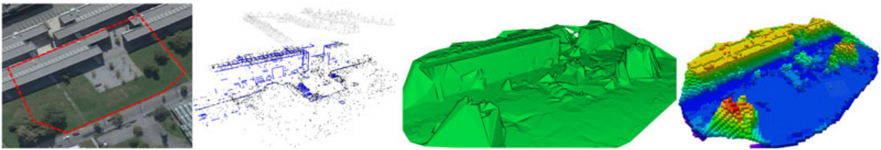
FIGURE 10 Scene1 —Obstacle map of size 105 \text{ m} \times 75 \text{ m} generated onboard in \approx 2.75 min from 56 images, from left to right: “Google Earth ©2015” image with red contour around the effectively mapped area, the SfM sparse model, the surface model, and the Octomap obstacle map with 1 m resolution. SfM: Structure from Motion [Color figure can be viewed at wileyonlinelibrary.com ]
