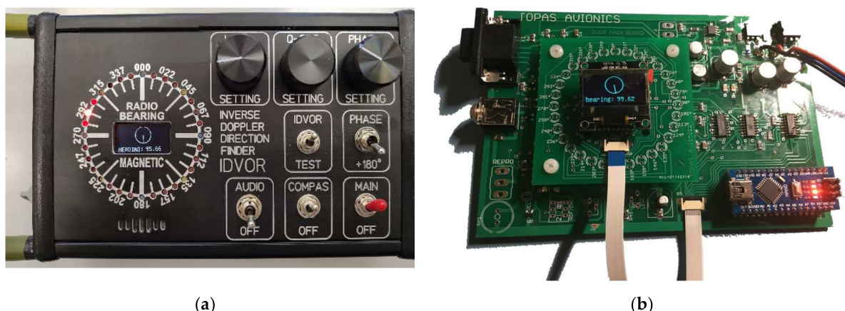
Figure 8. IDVOR control panel (a) and system board (b).
