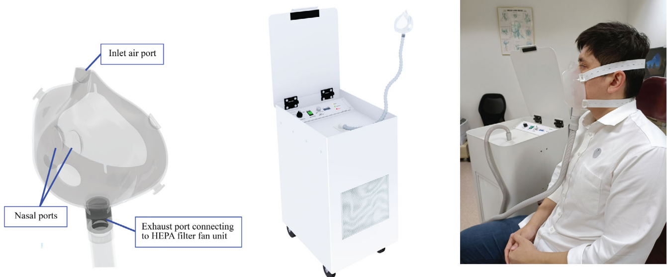
FIGURE 1 Prototype scope mask and filtration system (3D rendering and actual system)
