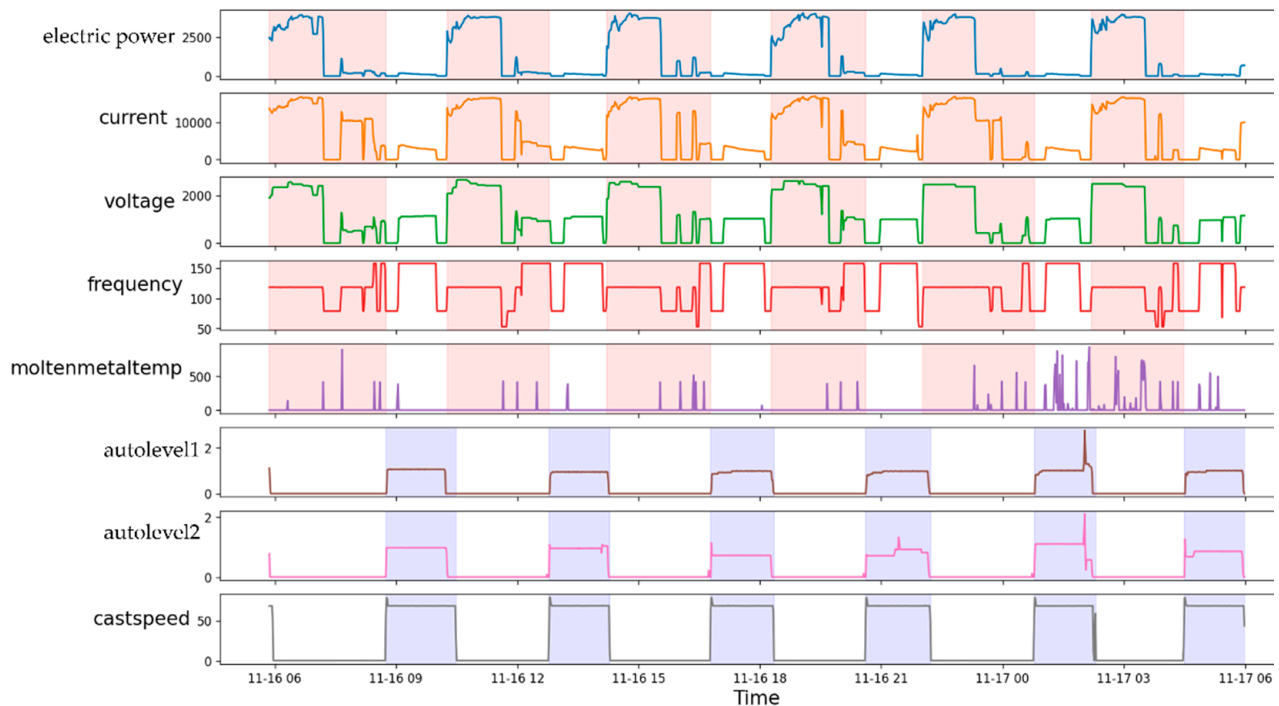
Figure 8. Extracting melting and casting TSWP from real-time data (pink areas indicate melting process, purple areas indicate casting process).
