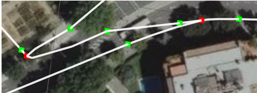
Figure 3. Detail of a sewer graph as used by our proposed localization method. The sewer galleries are marked in white lines. The manholes and forks are marked in green and red squares, respectively.
