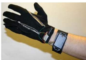
Figure 7. Sensorized glove connected to the measuring unit, which is fastened to the wristband.
