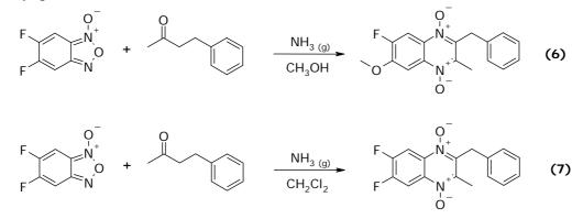
Finally, we observed another curiosity arising from the use of fluorinated compounds. When we attempted to prepare R7(R6)-fluorobenzofuroxan by oxidation of the corresponding fluoronitroaniline, as previously described [23], the compound obtained was actually R7(R6)-methoxybenzofuroxan. Once again, methanol was present in the reaction as solvent. Therefore R7(R6)-fluorobenzofuroxan was prepared by thermal decomposition as reported [22, 23, 24].
