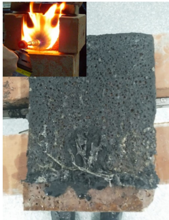
Figure 3. "Liquid wood" fire testing and "peeling effect" of burnt layers [55].
