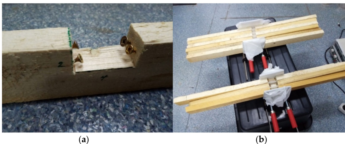
Figure 4. Wooden beams used in bending test: (a) wood screws installed in 2 \times 4 cm groove beam; (b) 2 \times 2 cm groove beams and 2 \times 4 cm groove beams clamped in separate stacks.
