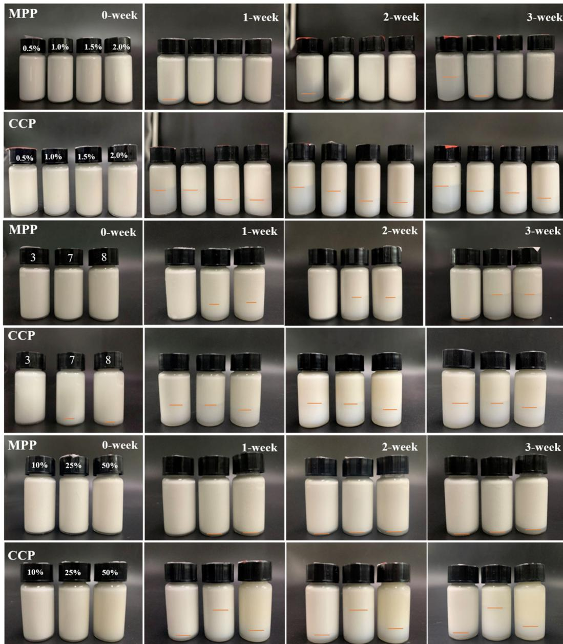
**Figure 4.** Macroscopic pictures of emulsions prepared by MPP and CCP over 3-week storage. A scanning light-scattering instrument was used to test the physical stability of the emulsion. Moreover, centrifugal determination and storage evaluation, assisted by the macro photos during the storage process, comprehensively evaluated the emulsion stability.
