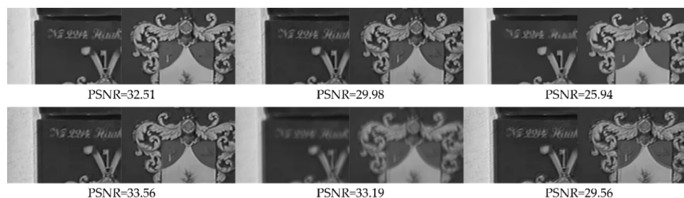
Figure 15. The effect of the restored first frame on the deblurred frame. Top: The restored first frames with different accuracies. Bottom: The corresponding deblurred second frames by our method.
