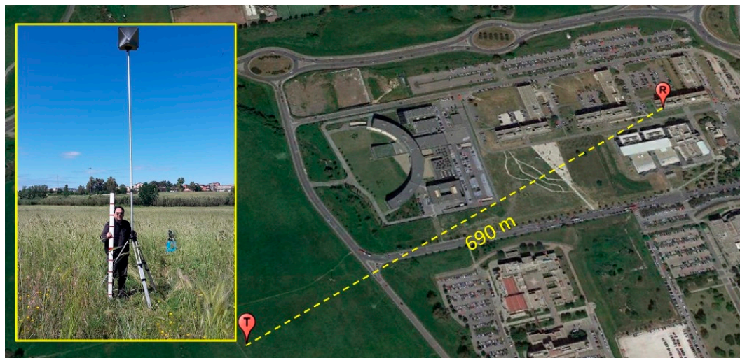
Figure 4. R and T denote the positions of the radar on the roof of the Information building ( 41^{\circ}51'6.40'' N, 12^{\circ}37'0.50'' E) and of the target ( 41^{\circ}51'6.40'' N, 12^{\circ}37'0.50'' E), respectively.
