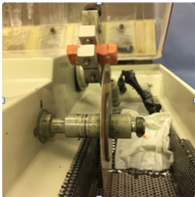
Figure 1 Low speed, double-sided diamond disk (ISOMET 2000 Precisions SAW).
