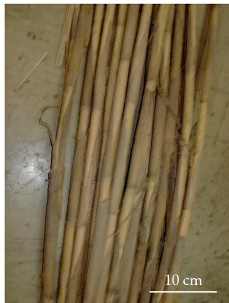
**Figure 1.** Giant reed used in the manufacturing of the panels.
