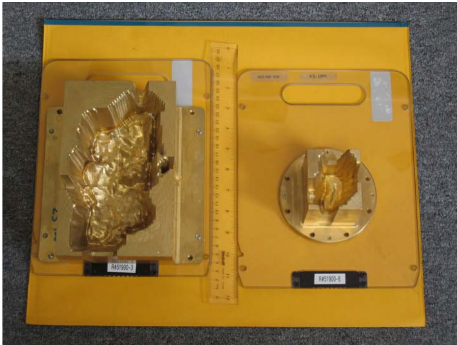
FIG. 1. Modulators from •Decimal mounted on the Siemens coded trays. One of the large compensators (11.3 kg) from the initial 7-field plan that did not require extensive blocking within the field is shown next to one of the 7-field IMRT modulators for prostate (1.8 kg).
