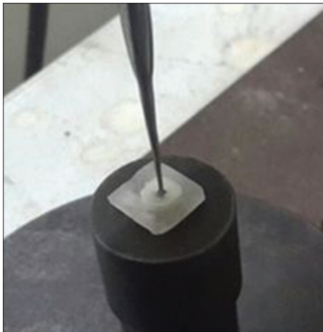
Figure 7: Push-out bond strength assessment using universal testing machine
