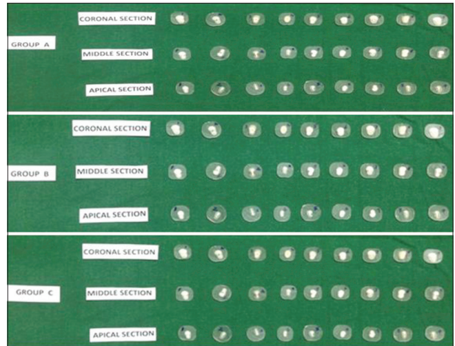
Figure 6: Labeling and grouping of sample for push-out bond strength assessment
