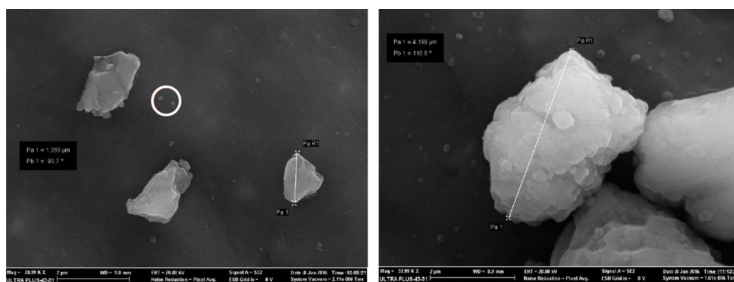
Figure 6. SEM analysis of the particles collected on 11 February 2015, during a drone launch exercise.
