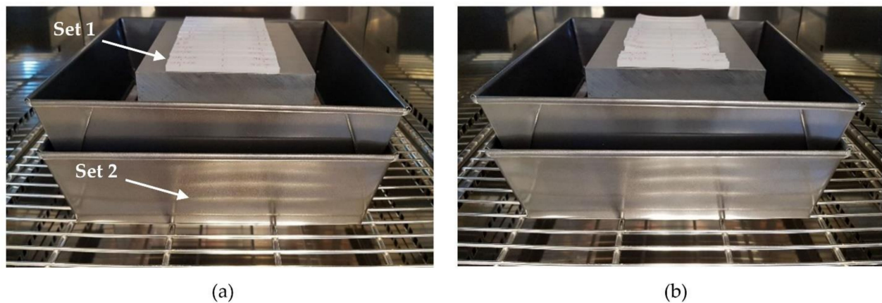
Figure 5. (a) Samples before thermal treatment in the furnace; (b) after thermal process, deformation is clearly visible in samples of Set 1.
