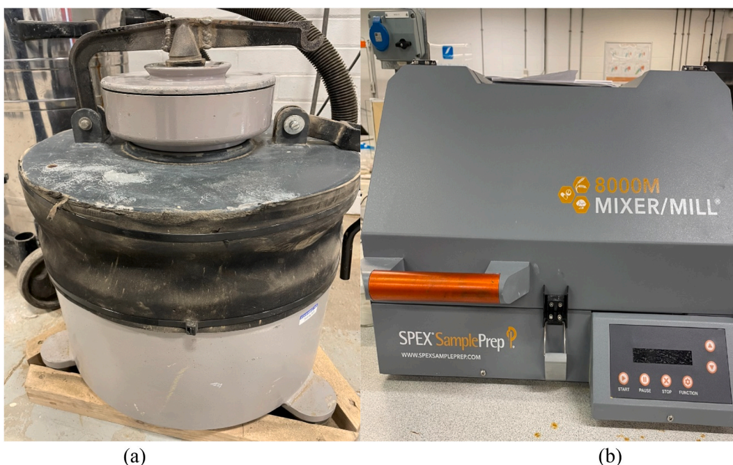
Fig. 13. (a) SIEBTECHNIK TEMA T1000 vibratory disc mill (b) An 8000 M Mixer/MILL ball grinning machine.
