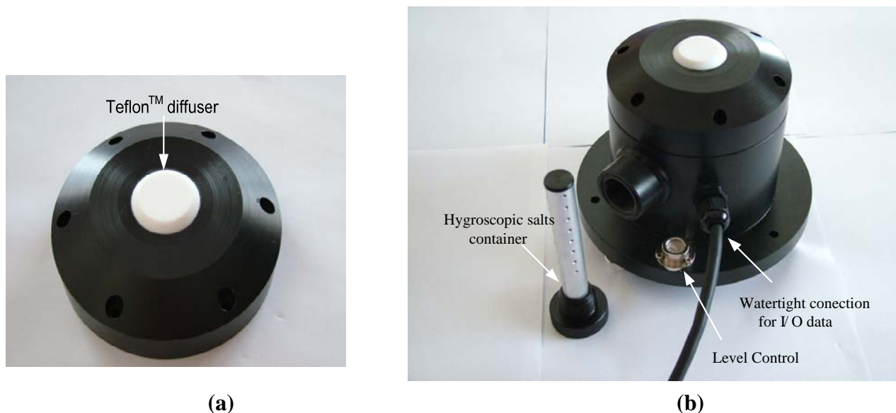
Figure 4. Developed pyranometer: (a) Detail of the diffuser in the pyranometer top. (b) Body of the pyranometer showing the container of hygroscopic salts and gauge level.
