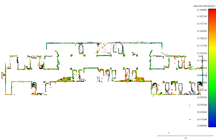
(a) Comparison between investigated LiDAR and ground-truth.
