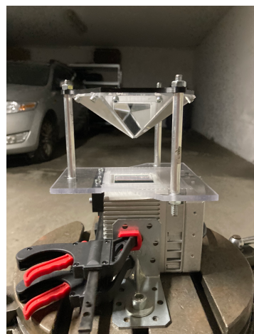
(a) Livox Mid-40 LiDAR with six planar reflectors.
