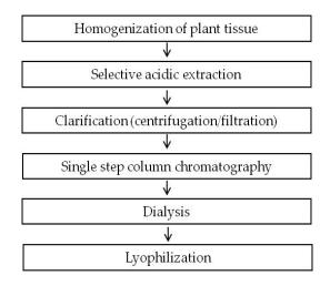
**Figure 1.** Flowchart of the experimental procedure for colicin purification from plant biomass by selective extraction, cation exchange chromatography, dialysis, and lyophilization.
