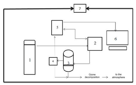
Scheme 1. Ozoniser used in experiments: (1) Oxygen source; (2) Ozone generator (BMT 803 N, BMT Messtechnik, Berlin, Germany); (3) Glass reactor with sintered glass G4; (4) drier (DH3, BMT Messtechnik, Berlin, Germany); (5) Ozone concentration meter (BMT 964, BMT Messtechnik, Berlin, Germany); (6) Regulatory system; (7) Monitoring ozone concentration in the laboratory (ECOZONE<sup>TM</sup>).
