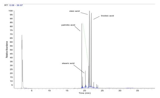
**Figure 1.** The GC-MS fatty acid profile of refined olive oil: Palmitic acid—Hexadecanoic acid, Stearic acid—Octadecanoic acid, Oleic acid—(9Z)-octadec-9-enoic acid; Linoleic acid—(9Z,12Z)-Octadeca-9,12-dienoic acid.
