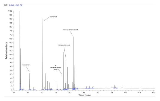
Figure 2. The results of GC-MS analysis of olive oil after ozonation (0.1 mole  $O_3/100$  g oil).
