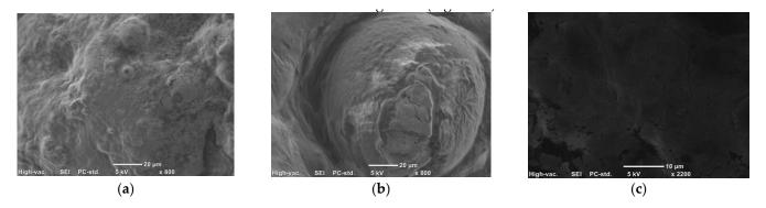
**Figure 5.** Homogeneity of emulsions based on different types of olive oil: (**a**) Refined olive oil; (**b**) Ozonated olive oil 0.04 mole  $O_3/100$  g oil; (**c**) 0.10 mole  $O_3/100$  g oil; Scanning-Electron Microscope JEOL JCM-6000.
