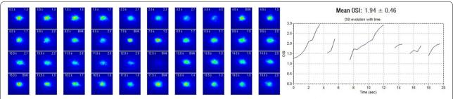
Fig. 1 The OQAS device records a 20-s examination with OSI measurement every 0.5 s. Image mode (left) presented the change in OSI over time. Line graph (right) provided the definite OSI evolution with time, whose data were analyzed from the left
