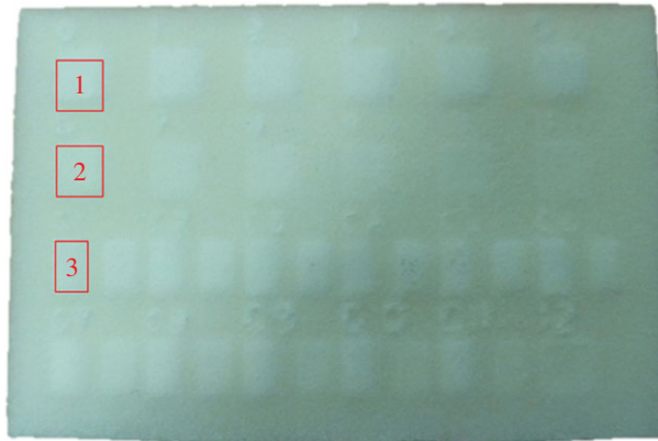
Figure 3. Measurement locations on the SLS sample with sub-surface regions of semi-consolidated powder. (Online version in colour.)
