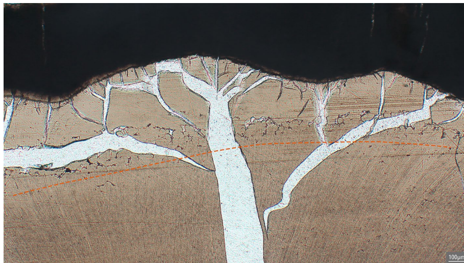
Figure 4. IGD in B61 (Grade 2) burned at 900 °C for 2 h, visible as a band of not fully fused calcospherites just above the dashed orange line. Note the heat-induced damage (white cracks) to the dentine (light brown).
