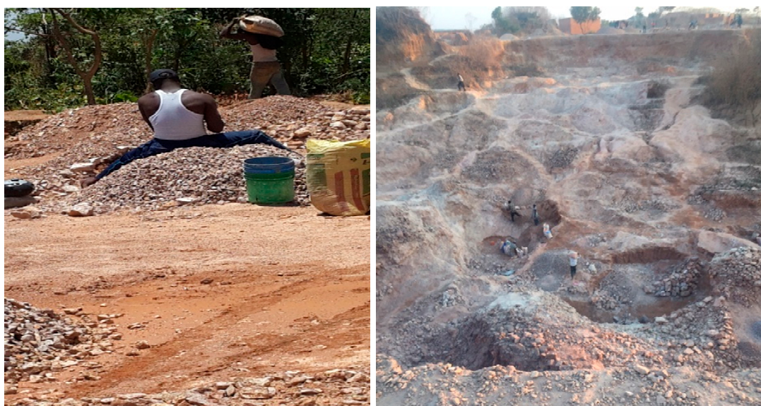
Figure 1. Left panel: An artisanal stone-crusher and a transporter of stones working in precarious conditions. Right panel: General view of the site where stones are manually extracted and then transported on shoulders towards the place where they are kept before being transformed into gravels that will be sold to the purchasers for building roads, bridges, houses.
