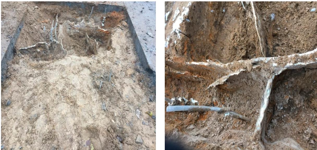
**Figure 2.** Different resin sections were distributed in the massive of the injected soil at a depth of 0.4 m [65,68].
