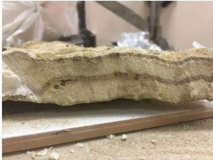
**Figure 1.** Resin samples were extracted from the injected plot after the injection process of the field investigations [67].
