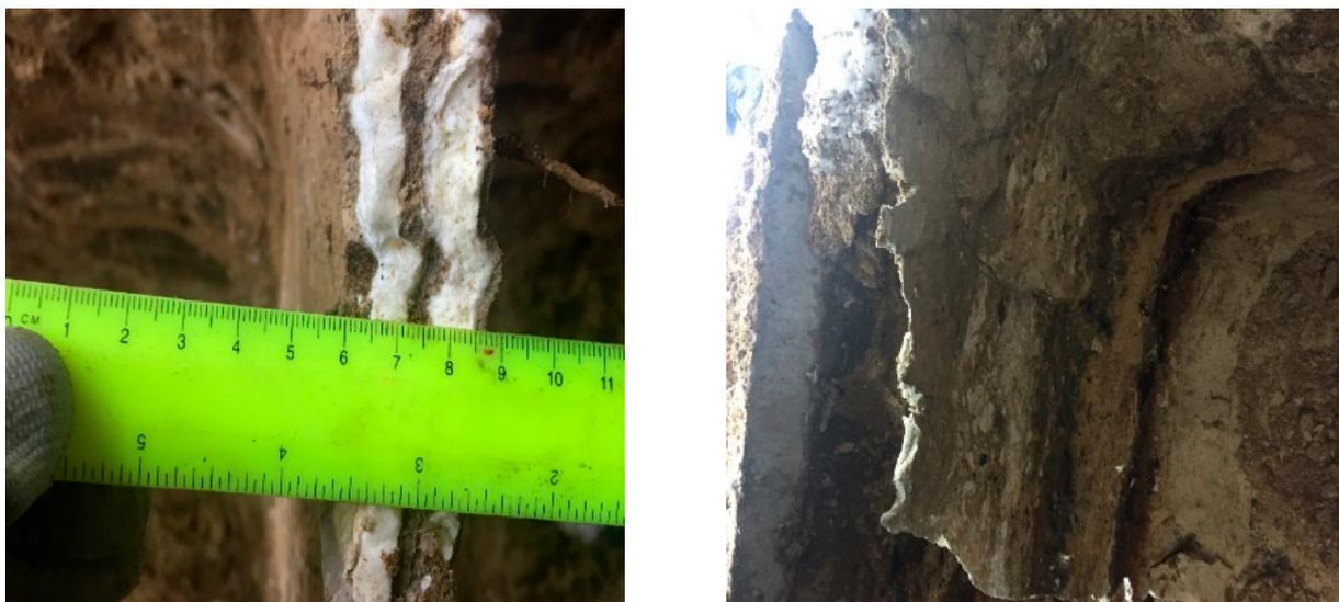
**Figure 3.** Different resin sections were distributed in the massive of the injected soil at a depth of 1.1 m [65,68].
