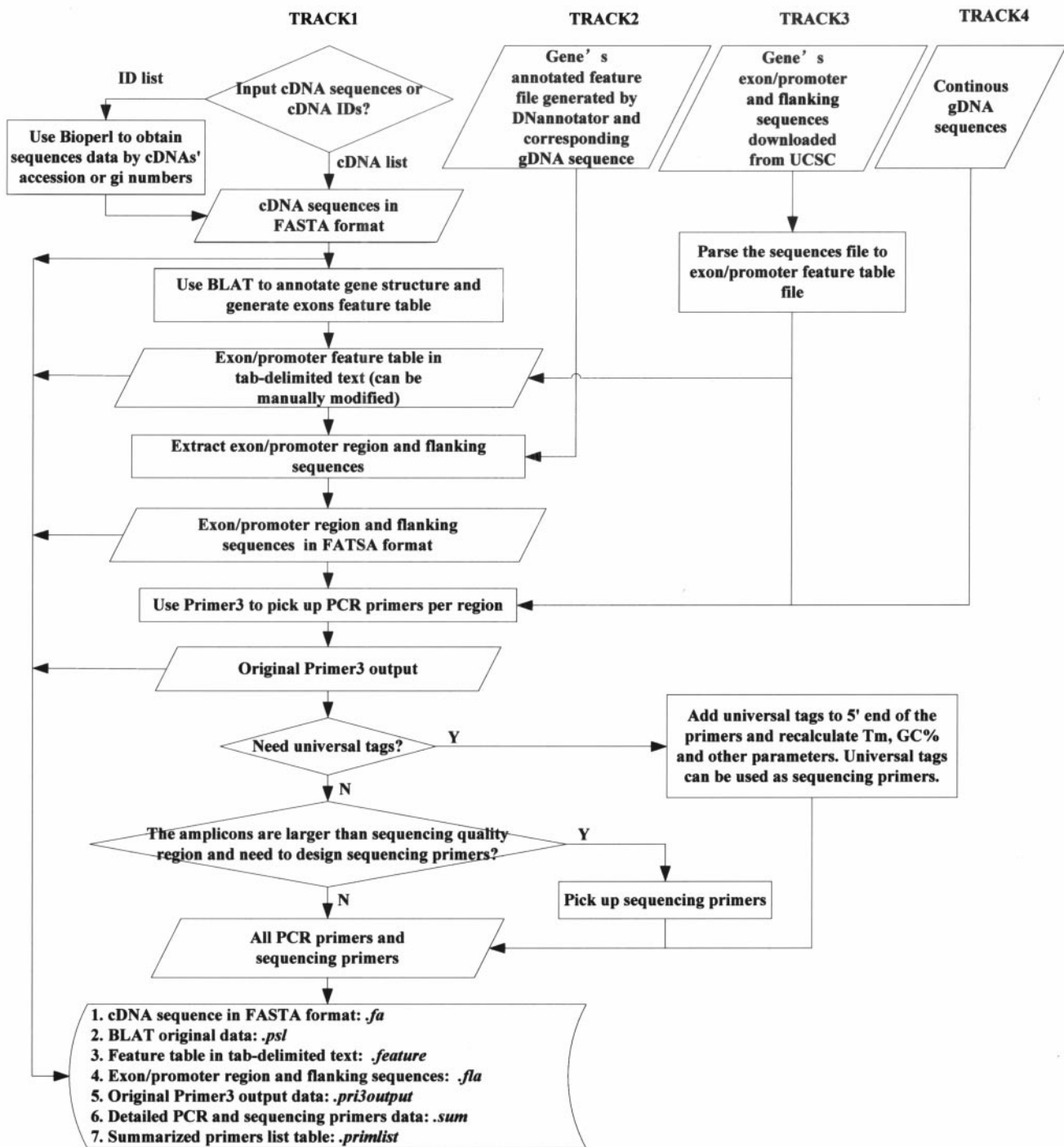
Figure 1. The workflow of MutScreener. Rectangles and rhombi show the processes that the program performs. Parallelograms show the data, either supplied by users or generated by MutScreener.
