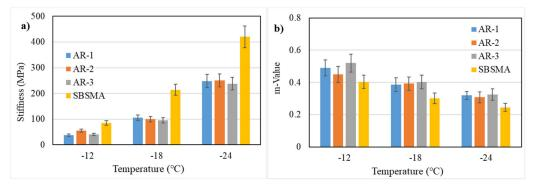
Figure 5. Stiffness and m-value in BBR tests. (a) stiffness; (b) m-Value.
