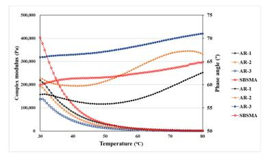
Figure 3. Results of temperature sweep.
