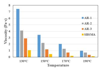
Figure 2. Results of Viscosity at 130 °C, 150 °C, 170 °C and 190 °C.
