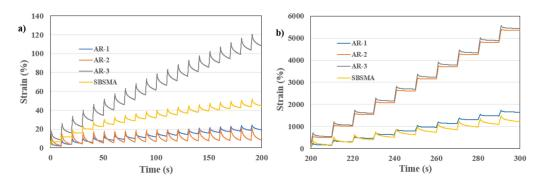
Figure 4. MSCR results at 64 °C. (a) load of 0.1 kPa; (b) load of 3.2 kPa.
