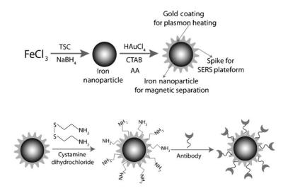
**Figure 1.** Popcorn shaped, magnetic core, gold shell nanoparticle synthesized and modified with an antibody. Reprinted with permission from ref [24]. Copyright © 2013 WILEY-VCH Verlag GmbH & Co. KGaA, Weinheim.
