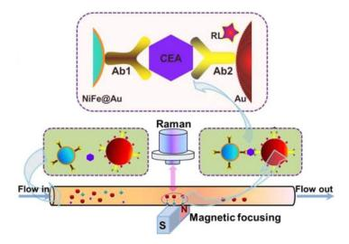
**Figure 4.** Illustration of SERS detection of cancer biomarker CEA (carcinoembryonic antigen). Using functional nanoprobes consisting of Au coated NiFe magnetic nanoparticles (NiFe@Au), capture antibodies (Ab1), detection antibodies (Ab2), and Raman labels (RL). Reprinted with permission from ref [101]. Copyright © 2015 American Chemical Society.
