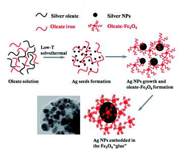
**Figure 2.** Magnetic Fe3O4 NPs and plasmonic Ag NPs forming an MPPs cluster. Reprinted with permission from ref [50]. Copyright © 2015 The Royal Society of Chemistry.
