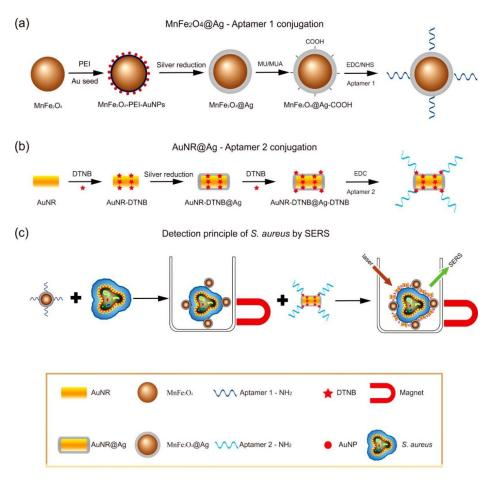
**Figure 3.** Scheme of Staphylococcus aureus detection by SERS using MPPs. (**a**) Synthesis of monodispersed silver-coated magnetic nanoparticles and their conjugation with aptamer 1; (**b**) Synthesis of gold core/silver shell plasmonic nanoparticles, labeled with SERS tag (DTNB), and their conjugation with aptamer 2; (**c**) operating principle for S. aureus detection. Reprinted with permission from ref [25]. Copyright © 2015 American Chemical Society.
