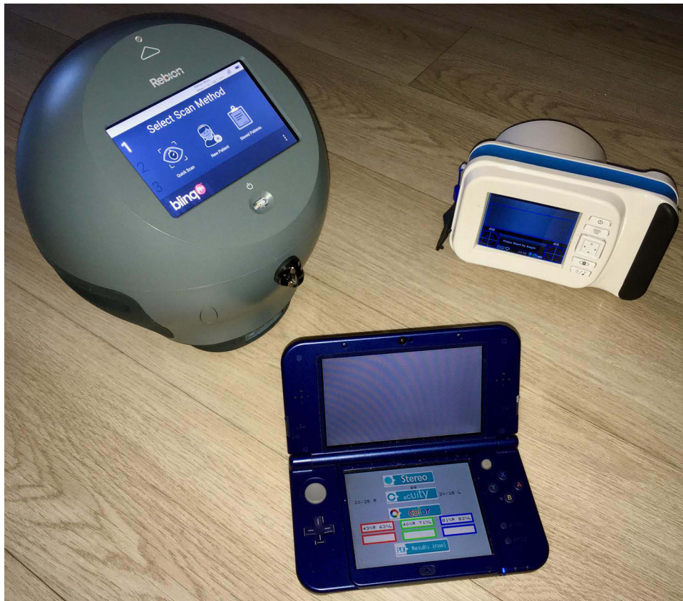
Figure 1 Three vision-screening devices: Rebron blinq birefringent binocular foveation scanner (upper left), Adaptica 2WIN infrared multiradial autorefractor (upper right), and PDI Check dynamic forced-choice vision-screening game on the Nintendo 3DS (bottom).
