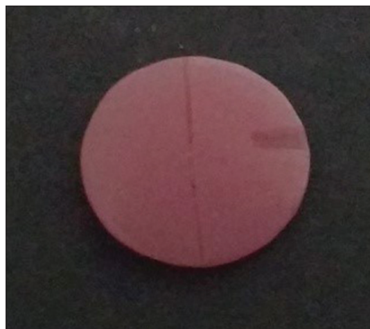
Figure 4: Small depression drilled on one side in sample disc
