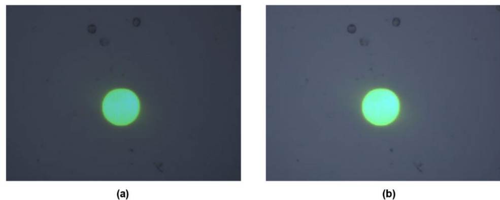
Figure 5. (a) Original cell image taken by CCD and (b) cell image with dark corners removed.
