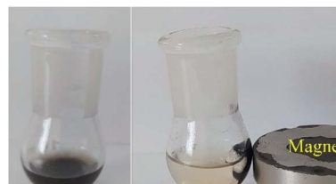
Fig. 8 Reaction mixture in the absence (left) and presence (right) of an external magnet.
