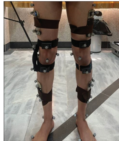
Figure 1: Placement of two inertial measurement unit sensors and the wearable device
