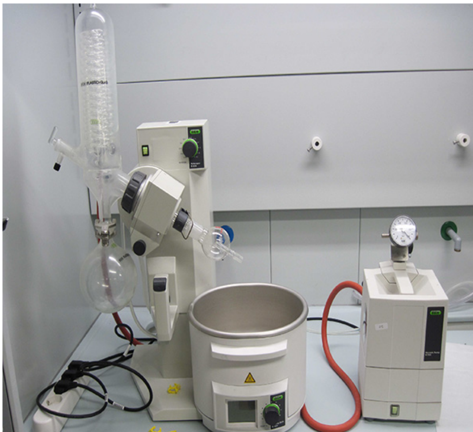
Figure 1. The rotary evaporator and vacuum pump. Click here to view larger image.
