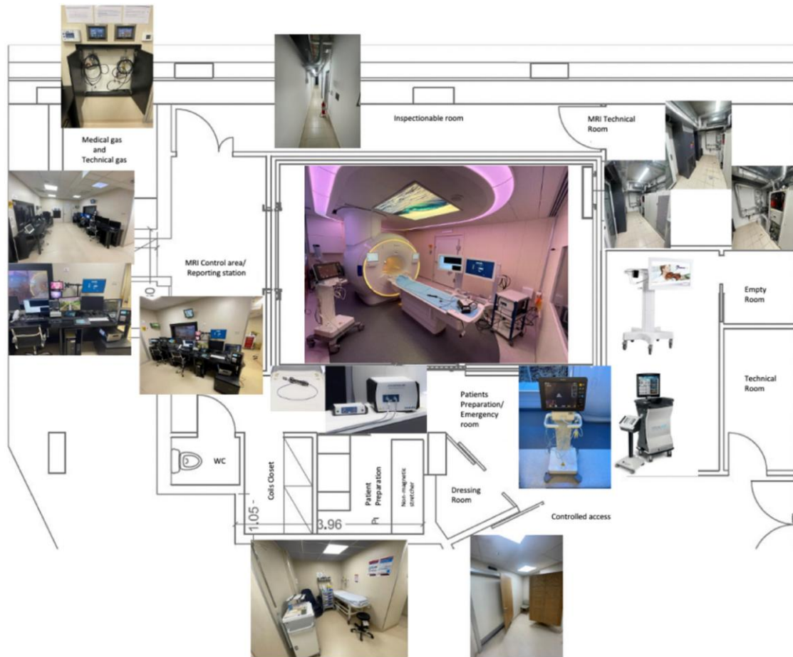
Figure 1 Map of the interventional MR department of policlinico casilino of Rome, Italy. At the centre of the picture, the scanner room. All around are present several technical rooms and the MRI cardiac ablation devices needed for the procedure.
