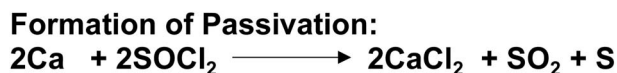
Fig. 2 Model for the formation of \text{CaCl}_2 passivation of the Ca metal in the \text{Ca}(\text{AlCl}_4)_2\text{-SOCl}_2 electrolyte.
