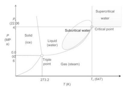
**Figure 3.** Phase diagram of water with marked sub- and supercritical region, where Pc represents critical pressure and T<sub>C</sub> critical temperature. Reprinted with permission from ref. [49]. Copyright 2016 Elsevier.
