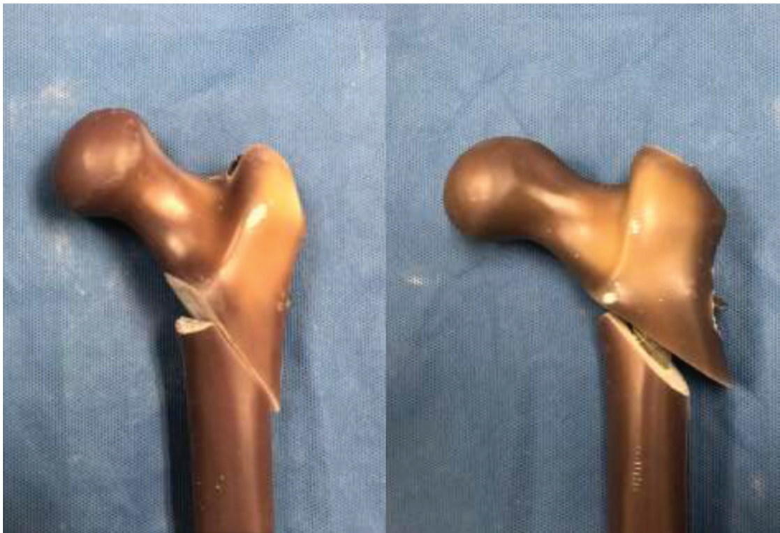
Figure 1. Clinical photograph of an anatomically reduced and a varus malreduced intertrochanteric OTA/AO 31-A3.1 (“reverse oblique”) fracture prior to testing.
