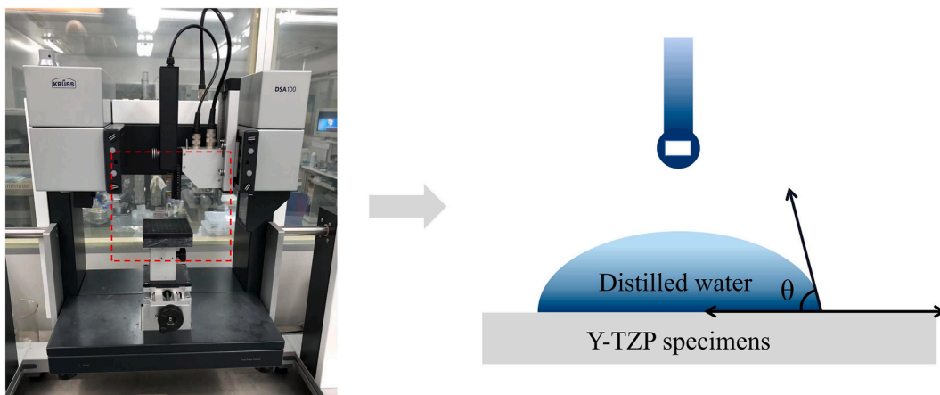
Fig. 3. The process of measuring contact angle.
