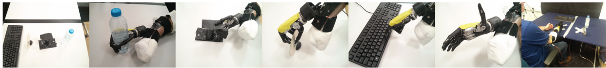
Fig. 3 Real-time control pick and place experiment. Participants were instructed to use a prosthetic hand to grasp and relocate three objects and finally press the 'space' key on a computer keyboard (left). Five grip types were used: power/cylindrical (water bottle), lateral (credit card simulator), tripod (CD), index finger pointer (computer keyboard) and hand open. A trial with an amputee participant is shown on the right
