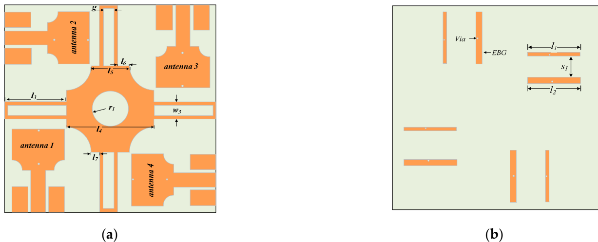
Figure 6. The geometry of the proposed MIMO antenna. (a) Front side (b) backside.
