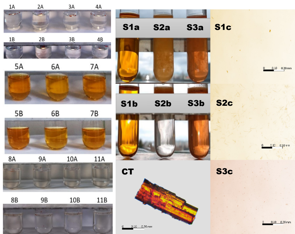
Figure 3. Left panel: macroscopic illustration of CT in various solvents and color intensity on the first (A) and eighth days (B) after dissolution in the solvents: distilled water (1), 0.1 mol/L sodium hydroxide (2), 1.0 mol/L sulfuric acid (VI) (3), 0.5087 mol/L hydrochloric acid (4), methanol (5), ethanol (6), isopropanol (7), AMPD (8), TRIS (9), TEOA (10), and TIPA (11). Middle panel: macroscopic illustration of CT in 96% ethanol (S1), 8% ethanol (S2), and 8% ethanol with a 0.1 mol/L solution of NaOH (S3). Illustration of the influence of ethanol on the solubility of CT in the 0.1 mol/L solution of NaOH immediately (a) and after 5 min (b), and a microscope image of the powdered CT particle in the air. Right panel: microscope images of a drop taken from the surface of the samples in the test tubes S1b, S2b and S3b, respectively. The bar represents the same longitude (200 \mu\text{m} ). The details are in the text.
