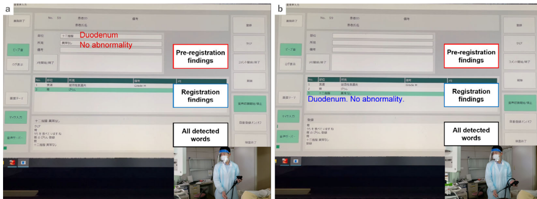
Figure. Speech recognition (SR) system workflow. All words spoken by the endoscopist were displayed in the “All detected words” section at the bottom of the screen. The recognized findings were first displayed in the “Pre-registration findings” section at the upper part of the screen (a). When the proper findings were displayed, the endoscopist used the command “Register” to finalize the findings in the center of the screen as “Registration findings” (b).
